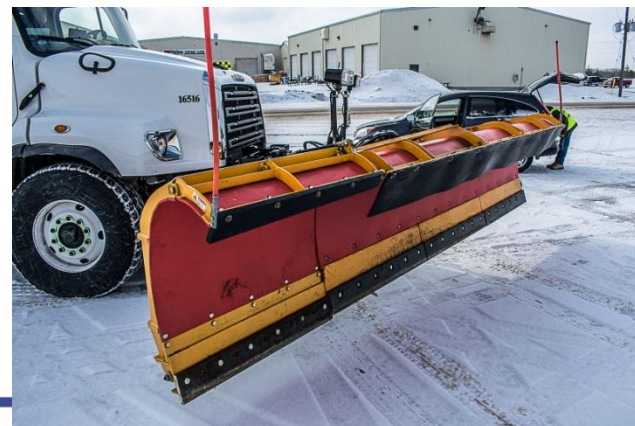
Extension fully deployed for seamless moldboard
